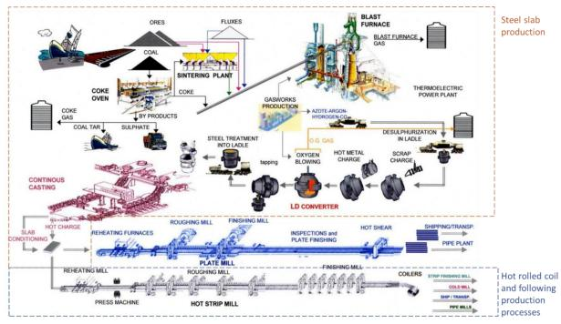
Figure 1: Steel slab and hot rolled coil production in Taranto plant, necessary for the Cold rolled and Annealed coils
