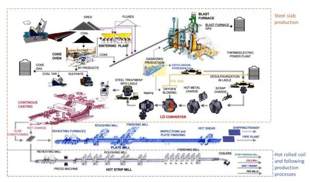
Figure 1: Steel slab and hot rolled coil production in Taranto plant, necessary for the Hot dip galvanized coils
